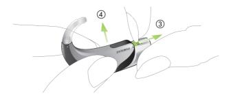
Pull the hearing system upwards with the other hand (4).
