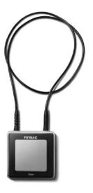
iCom is also capable of transmitting a stereo audio signal from any Bluetooth (or via a standard audio jack) enabled device such as MP3 players, laptops, computers and televisions.
