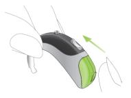
Close the battery compartment. Your Naída hearing systems are always working in the initial hearing program, and at the preset volume when turned ON.
