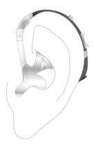
Check the placement of the earmold by tracing the contour of the ear with your finger.
