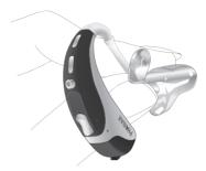
Using the hand on the same side you wear your hearing system, grasp the earmold between the thumb and index finger.
