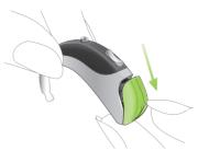
Using the nail grip, slightly open the battery cover until it snaps to its OFF position. Keep in mind that Naída hearing systems are water resistant (sealed) and need a slightly stronger force to the OFF position.
