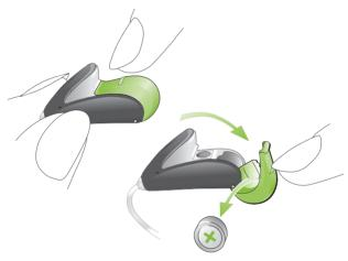
Remove the protective foil from the new battery. Wait for at least 30 seconds before inserting it.
