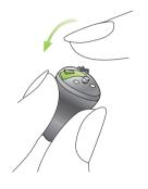
The hearing system is switched ON when the battery compartment is closed. Your hearing system is automatically set at your preferred volume and in your default hearing program.
