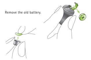
Remove the protective foil from the new battery.
