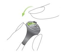
Handle the battery compartment gently and do not use excessive force.
