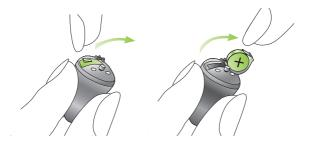
Do not try to open the compartment further than shown in the drawing.
