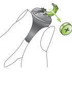
Remove the protective foil from the new battery.
