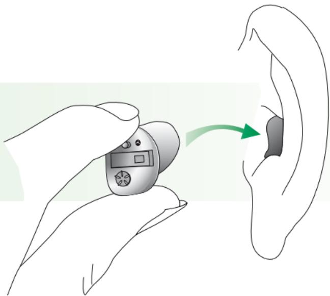
Grasp the hearing system between the thumb and index finger, using the hand on the same side you wear your hearing system. Insert it canal end first into the ear canal. Tug gently on your ear lobe and push the hearing system into the correct position.
