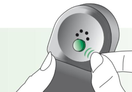
Hold the telephone handset nearly vertically, similarly to making a telephone call. Hold the magnet near to the "listening end" of your telephone handset and release it. The magnet will automatically flip to the correct side at the right location.
