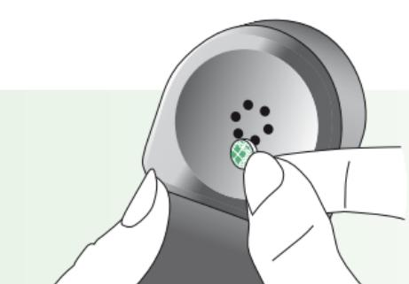
Use the double sided adhesive tape to stick the magnet to the location described before (see pictures). Do not cover the sound openings of your handset. Make sure the magnet is safely fixed to the "listening end" of the telephone handset.
