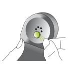
Clean the telephone handset thoroughly. Hold the telephone handset nearly vertically, similar to making a telephone call. Hold the magnet near to the "listening end" of your telephone handset and release it. The magnet will automatically flip to the correct side.
