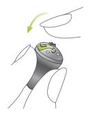
The hearing system is switched ON when the battery compartment is closed. Your hearing systems are automatically set at your preferred volume and in your default hearing program.
