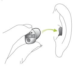
Grasp the hearing system between the thumb and index finger, using the hand on the same side you wear your hearing system. Insert the canal end into the ear canal. Tug gently on your ear lobe and push the hearing system into the correct position.
