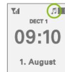
**Ring tone off:** Press the
