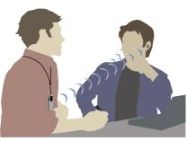
Speaker talking into Hearing instrument the transmitter user wearing FM receiver(s)
