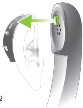
Instead of holding the phone against your ear canal hold the earpiece of the phone against the microphone, which is at the front of your hearing system.
