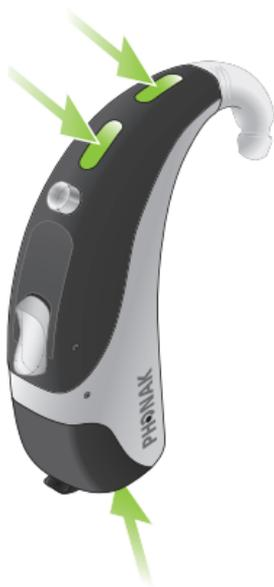
The life span of the Wind and Weather Protectors should be up to several months, depending on the environment (humidity, dust, perspiration, etc.). The Wind and Weather Protectors should not be cleaned but replaced regularly.
