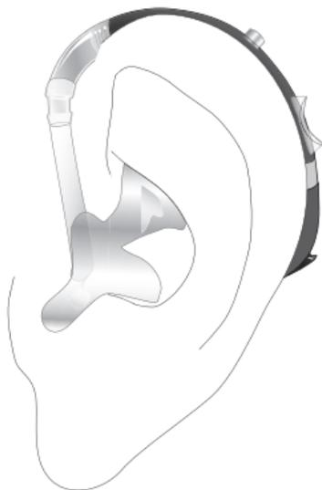
Check the placement of the earmold by tracing the contour of the ear with your finger.
