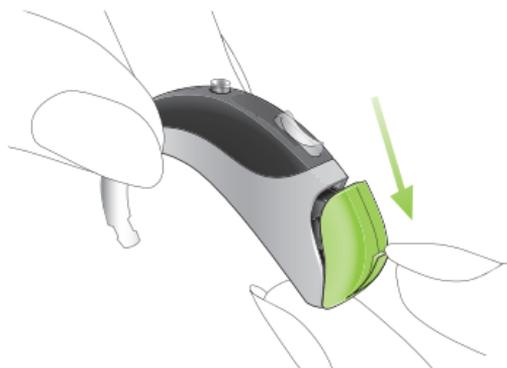
Using the nail grip, slightly open the battery cover until it snaps to its OFF position. Keep in mind that Naída hearing systems are water resistant (sealed) and need a slightly stronger force to the OFF position.
