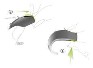
Battery compartment lock has the same functionality with FM (5)
