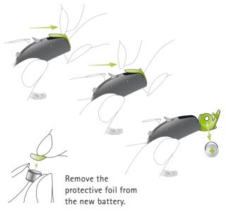
Insert the new battery with the "+" sign (flat side of the battery) in line with the "+" marked on the battery compartment and close it.
