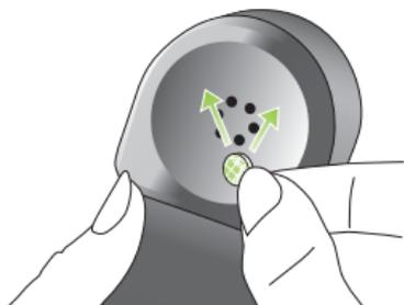
If you hold the telephone receiver in your **left hand** when making telephone calls, position the magnet in the **upper left half** of the receiver.
