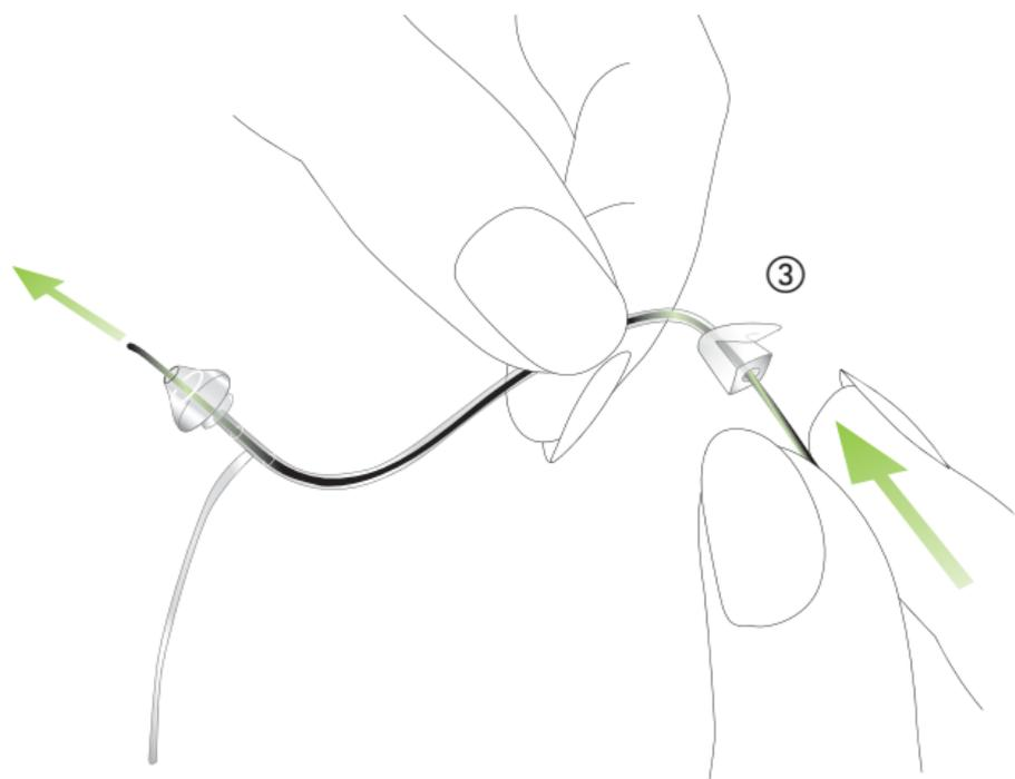
Insert the cleaning rod where the micro tube attaches to the hearing instrument and push it all the way through the micro tube and out through the dome or SlimTip ③. After cleaning it is important to remove the cleaning rod.
