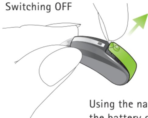
Using the nail grip, slightly open the battery compartment until it snaps to its OFF position.
