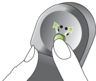
If you hold the telephone receiver in your **right hand** when making telephone calls, position the magnet in the **upper right half** of the receiver.
