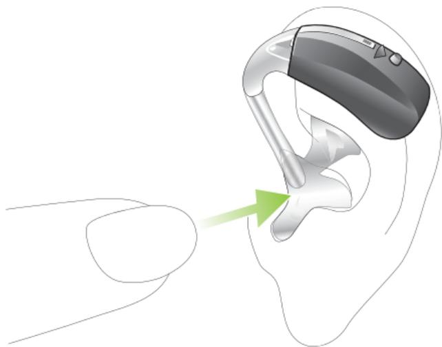
Place the canal portion of the earmold inside your ear canal. If it is difficult to get it into place, stretch your ear by pulling it gently backwards and upwards with your other hand. When the canal portion is in place, twist the earmold backwards so that it fits into the bowl part of your ear and the helix portion is under the fold.
