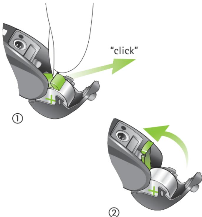
The battery can only be inserted when the latch is open (3). Move the latch over the inserted battery so that it lies against it (4). Lock the battery by pushing the latch towards the hearing instrument with your finger until it "clicks" into its final position (5). Before you close the battery compartment, check that the latch is locked in position and the battery can't be removed.
