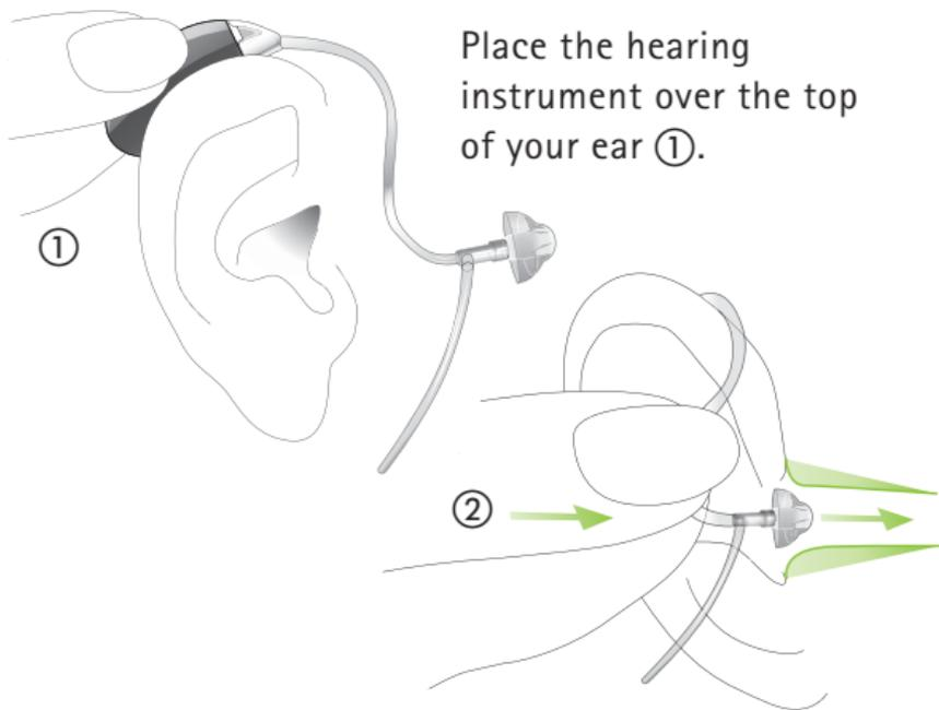
Hold the micro tube where it attaches to the dome or SlimTip ② and gently push the dome or SlimTip into your ear canal. The dome or SlimTip should be placed far enough into the ear so that the micro tube lies flush with your head.
