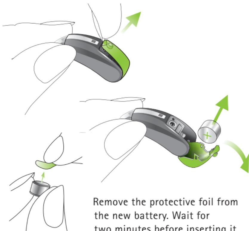
Insert the new battery with the "+" sign (flat side of the battery) as shown below. The correct battery orientation can also be seen on the inside of the battery compartment. Close the battery compartment.
