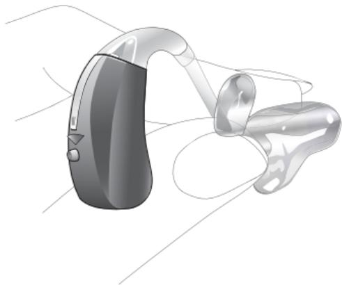
Using the hand on the same side you wear your hearing instrument, grasp the earmold between the thumb and index finger.
