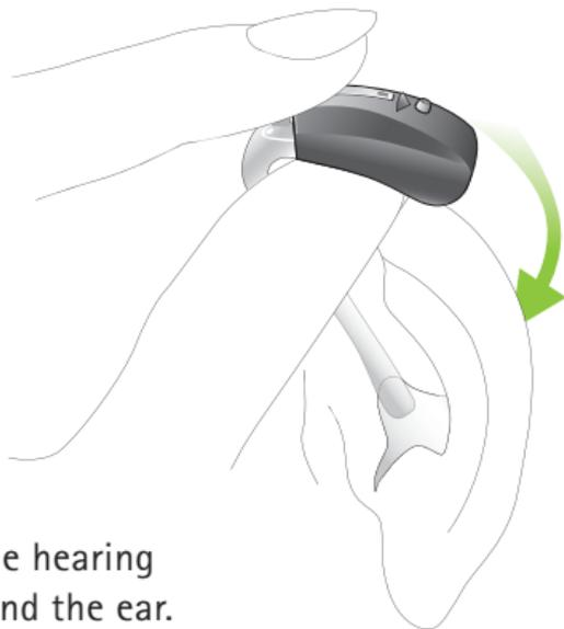
Now position the hearing instrument behind the ear. Be careful not to twist the tubing.
