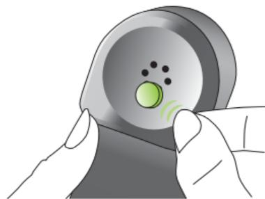
Clean the telephone handset thoroughly. Hold the telephone handset nearly vertically, similar to making a telephone call. Hold the magnet near to the "listening end" of your telephone handset and release it. The magnet will automatically flip to the correct side.
