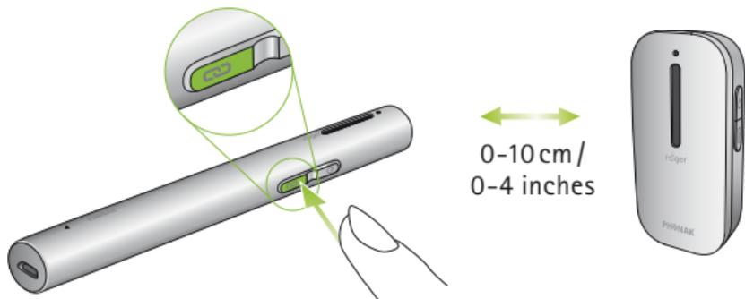
4. The indicator lights of both microphones will turn green for two seconds to indicate successful connection.
