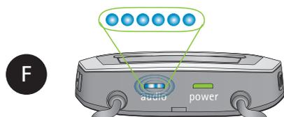
The audio indicator light will rapidly flash blue. As soon as BT300 indicator light turns solid blue, the pairing process is finished.
