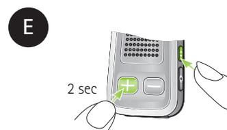
Switch your ComPilot on and push both buttons as shown for 2 seconds to start the pairing process.
