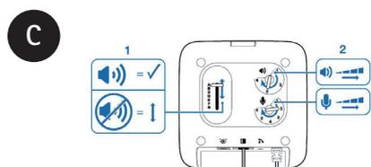
Ensure the configuration slide switch (1) is set to "A", the listening volume (2) is set to 3 and the speaking volume is set to 2 on the bottom of the MDA200.
