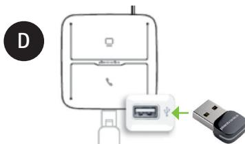
Ensure the BT300 adapter is fully inserted into the USB port of the MDA200. The indicator light of the BT300 will flash blue after approx. 10 seconds.
