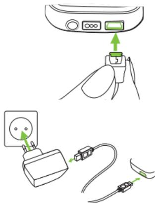
The power indicator is red during charging and will turn green when charging is complete.
