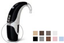
**ML10i** is a tiny Dynamic FM receiver for Phonak UltraPower hearing instruments that use a 675 battery.
