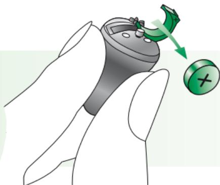
4) Insert the new battery. Please ensure that the "+" sign on the battery (flat side) is on the same side as the "+" sign on the battery cover.
