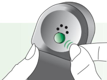
Hold the telephone handset nearly vertically, similar to making a telephone call. Hold the magnet near to the "listening end" of your telephone handset and release it. The magnet will automatically flip to the correct side at the right location.
