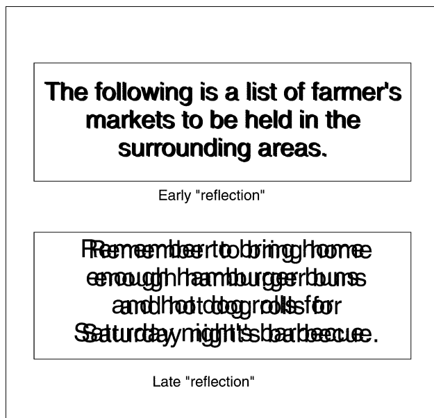
Figure 2. A simulation of the different effects of early and late reflections.
