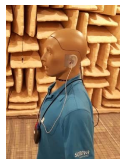
Figure 3: KEMAR set up in anechoic chamber for polar plot measurement
