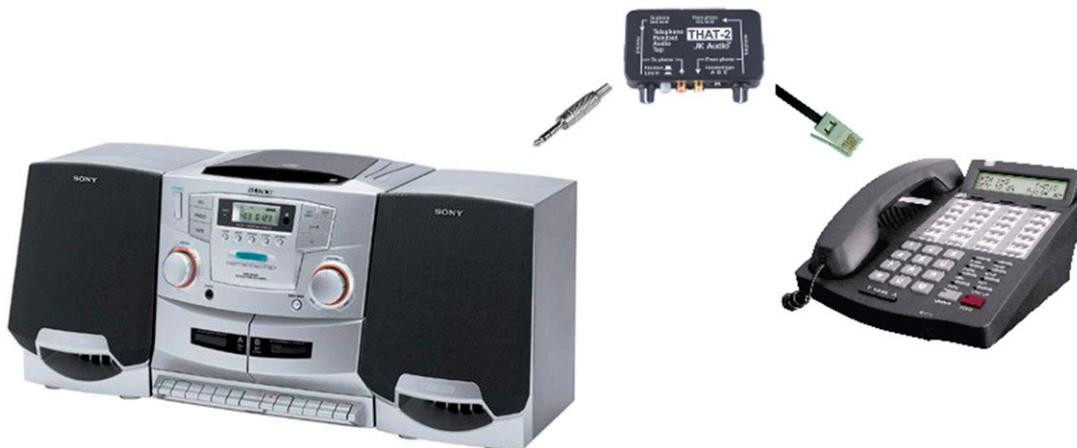
**Figure 4.** Sony compact disc player connected to a landline telephone via a THAT-2 telephone interface in order to allow for presentation of recorded speech materials.
