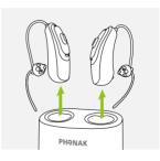
(i) Do not hold the tubes for removing the hearing aids from the charger as this can damage the tube.
