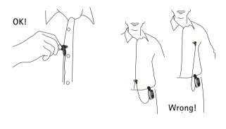
i Do not cover either of the two microphone openings!
