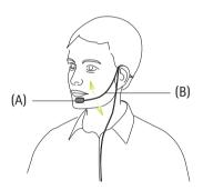
Make sure the head of the microphone is well positioned, as depicted above (A). If required you can easily bend the boom section (B).
