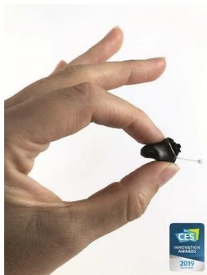
The Phonak Virto B-Titanium is the world’s first 3D-printed titanium hearing aid designed and engineered with ultimate discretion in mind. The shell is made of medical grade titanium, making it 15x stronger, 50% thinner, and up to 26% smaller compared to standard acrylic shells. A thinner shell gives 3D modelers more real estate for electrical components and venting. It also enables a deeper placement in the ear canal, resulting in a virtually invisible fit.
