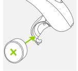
2. Place battery in the battery door with the "+" symbol facing upwards.
