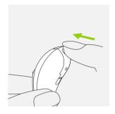
The battery is only tamperproof when the battery door is closed correctly. Always check after closing, that the battery door cannot be opened by hand.
