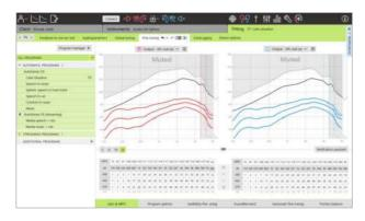
Fine tuning gives access to more specific fitting functionalities such as adjusting gain and MPO, as well as hearing performance and sound cleaning features, for an individualised fitting. Here you can access the Verification assistant to streamline your REM and test box measurements.
