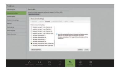
To perform a listening check and verify the mechanical function of ActiveVent, go to [Measurement settings] under [Trial & tools], located outside the client session. There are two measurements to choose from in order to verify each ActiveVent states, open versus closed.
