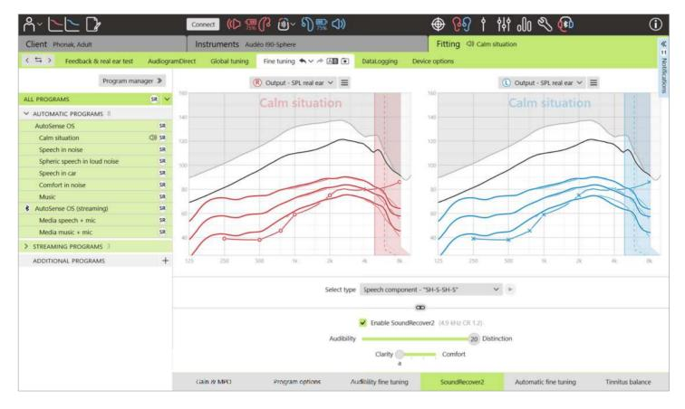
SoundRecover2 is a frequency compression system with adaptive behavior.
