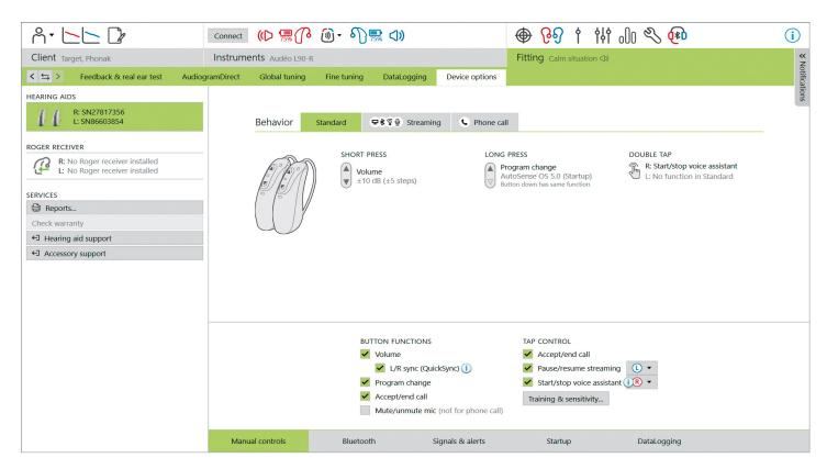
By clicking [Device options] you can configure hearing aid options such as manual controls, signals and alerts, startup behavior or DataLogging. For an overview of the multifunction button and Tap Control behaviors in different listening situations, click on [Standard], [Streaming] or [Phone call].
