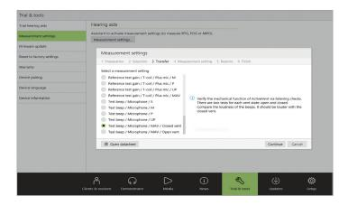
When performing the measurement for each vent status, you will hear a tonal signal and can compare the loudness of the signal between the open status and the closed status. You should expect the signal to be louder when it is played via the closed status. This would indicate the mechanical function of ActiveVent is working as expected.
