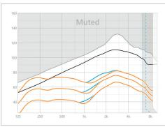
Looking at the direct sound compensation effect within [Output-SPL realear] will show that this small deviation is necessary for the purpose of sound quality improvement, such as preventing the client's own voice from sounding "hollow" or "echoey".
