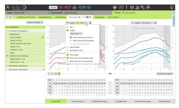
Target offers several curve display options to choose from. Each option offers a different view of how amplification is provided by the hearing aid, and can further support in the fine tuning process, depending on your fitting objectives. Below are the descriptions for each view.
