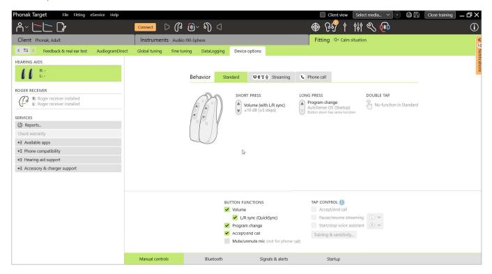
By clicking [Device options] you can configure hearing aid options such as manual controls, signals and alerts, startup behavior or DataLogging. For an overview of the multifunction button and Tap Control behaviors in different listening situations, click on [Standard], [Streaming] or [Phone call].
