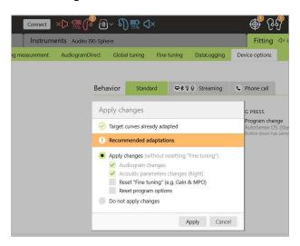
When a change is made that affects the amount of gain needed for the hearing loss, the target curves are automatically adjusted. This is for all fitting formula.
