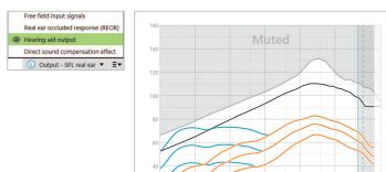
To convert the view to another scale, select [Output-HL] or [Output - SPL real ear], or [Gain - insertion gain] or [Gain - real ear].
