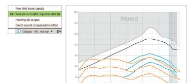
REOR: select [Output - HL] or [Output - SPL real ear] display. REOG: select [Gain - insertion gain] or [Gain - real ear] display.
