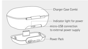
micro-USB connection to external power supply
