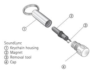
To be able to use the SoundLync, unscrew the magnet from the keychain housing and hold it inside
