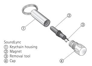
To be able to use the SoundLync, unscrew the magnet from the keychain housing and hold it inside the ear canal without touching the hearing aid.
