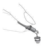
Note: Lyric can be removed using a blunt-nosed tweezer if the removal tool is not available. Use the tweezer to grasp the handle on the hearing aid and gently remove the hearing aid using a circular motion. This requires the help of a family member or friend. Please be especially careful if you are not removing the hearing aid yourself and advise the person helping you to work slowly in a circular motion when removing Lyric.
