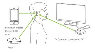
\* The TV Connector can be connected to any audio source such as a TV, PC or hi-fi system.
