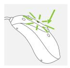
If the hearing aid is paired with a Bluetooth<sup>®</sup> enabled phone, a short press on the upper or the lower part of the button will accept an incoming call and a long press will reject an incoming call – refer to chapter 13.
