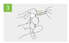
**2.** Pick up the new wax filter by inserting the slotted end of the changing tool.
