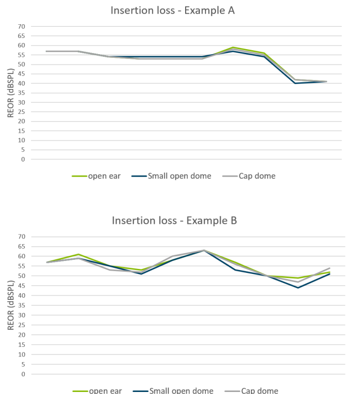
Figure 4: Measured real ear responses unaided (green) and occluded with a small open dome (blue) and cap dome (gray)
