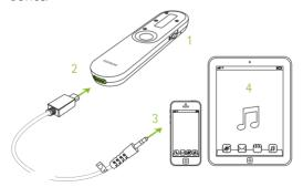
(j) Your Roger microphone will automatically mute when you plug in the audio cable. You can activate the microphone by pressing the center touch key. Now you will hear the audio device and microphone in parallel.
