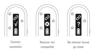
① Connecting a receiver is only required once. The hearing aid / Roger receiver will remain connected with your microphone even after the hearing aid / Roger receiver has been restarted.
