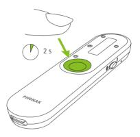
The muted microphone is indicated by a crossed microphone icon on the display. To unmute the microphone again, press and hold the function button again for two seconds.
