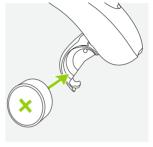
Place battery in the battery door with the "+" symbol facing upwards.
