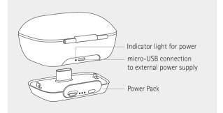
micro-USB connection to external power supply
