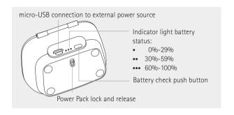
**3.** To check the remaining battery capacity of the Power Pack, press the battery check push button. The indicator lights will show the status.
