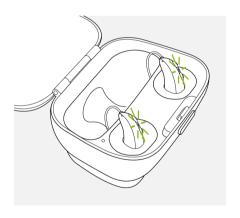
The charging process will automatically stop when the batteries are fully charged, so the hearing aids can be safely left in the charger. It can take up to 3 hours to charge the hearing aids. The charger cover can be closed while charging.
