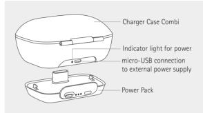
micro-USB connection to external power supply
