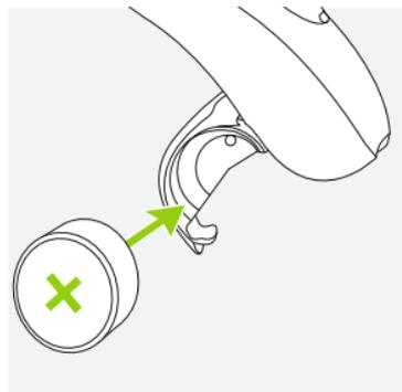
2. Place battery in the battery door with the "+" symbol facing upwards.
