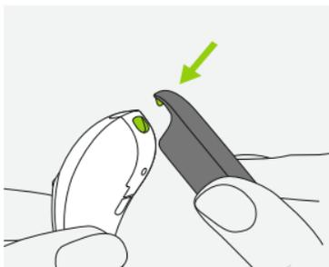
**1.** Place the tip of the tool in the small hole at the bottom of the hearing device.
