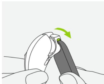
**2.** Use the tool as leverage to open the battery door by pulling the door with the tool in the direction of the green arrow.
